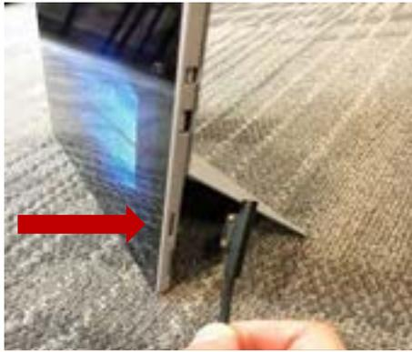
e. Plug the power supply into an electrical outlet. The LED on the charging cord should light up to indicate normal charging.
